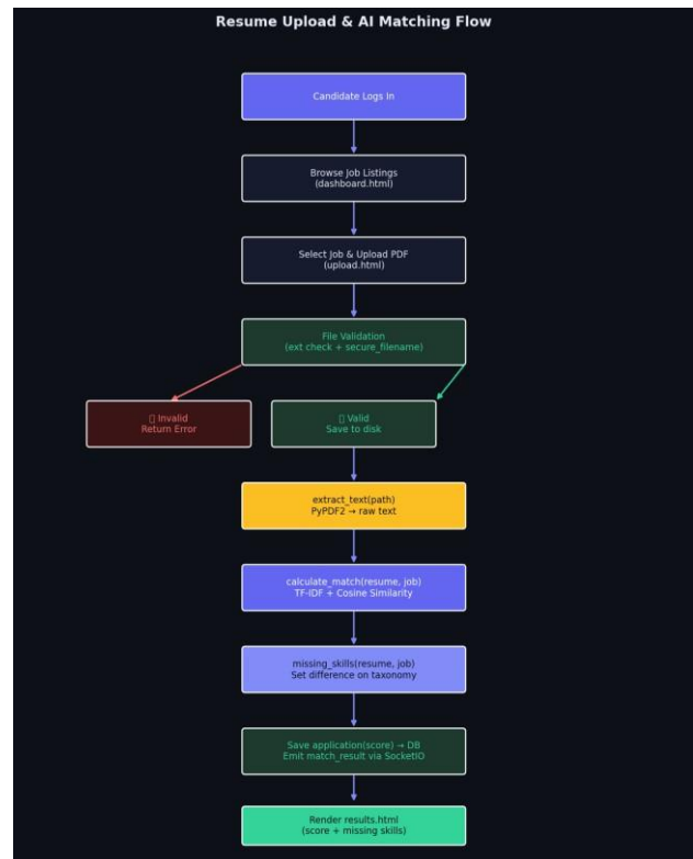
Figure 3: Resume Upload and AI Matching Flow — from login to results rendering
