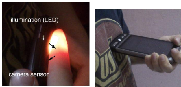
(a) PPG sensor. The camera records the micro-oxidation of the fingertip. The LED phone is positioned near the heart illuminates the fingertip in order to for better signal. produce a better signal.
