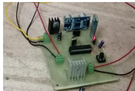
Fig.6 PCB with ultrasonic sensor, driver IC and Microcontroller
