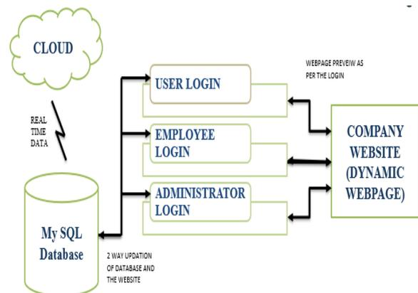
Fig 12: The block diagram showing the working principle of the Dynamic website of the system
