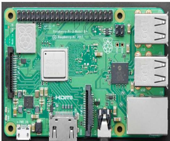
Fig9: Raspberry pi 3 B+ Module
