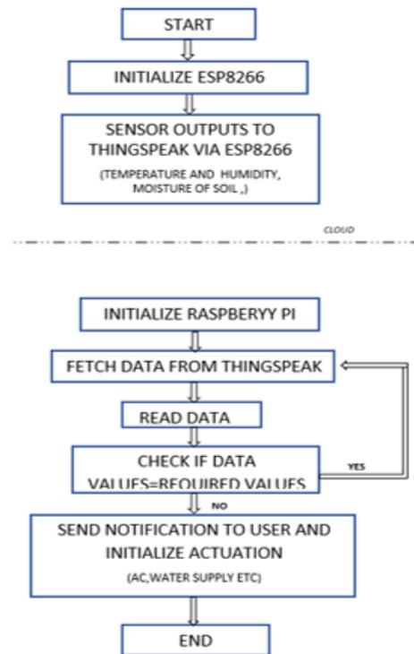
Fig7: Flow Diagram of the working of the sensing Node and Storing the value to the cloud.
