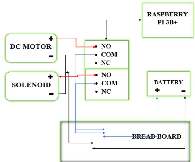
Fig 11: Circuit diagram for solenoid operation
