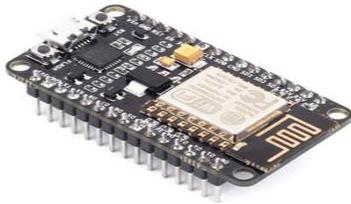
Fig3: Esp8266 controller
