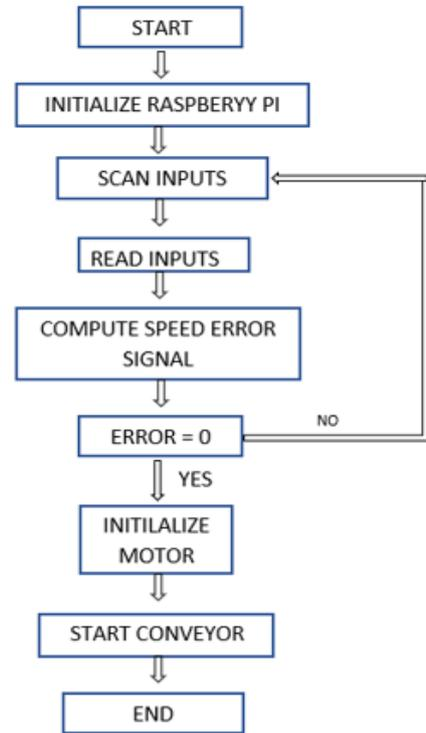
Fig 13: flow diagram of working of the conveyer belt system
