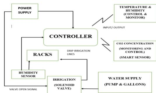
Fig 2: Sensing Node block diagram
