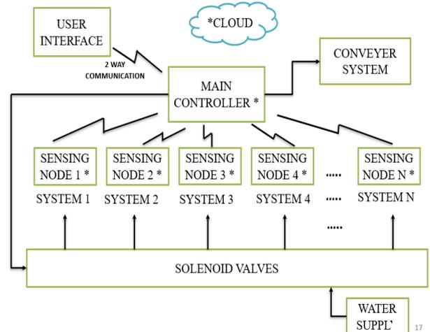
Fig 8: IoT system Block Diagram
