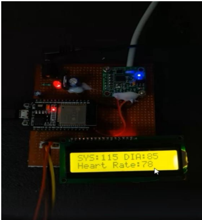
Figure 11. Heart rate and blood pressure sensor details are displayed on LCD Display
