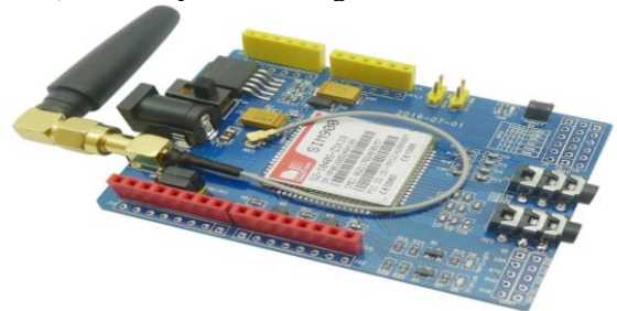
Figure 5, GSM SIM 900 shield for Arduino
