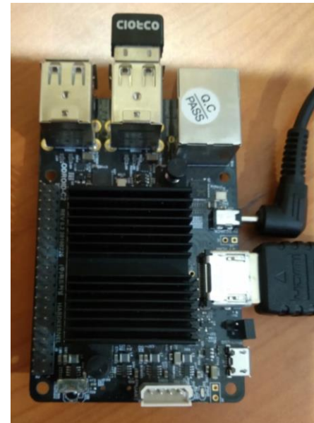
Fig2: Odroid-C2 after making all the respective connection
