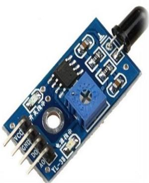
A sensor that is maximum touchy to a ordinary mild is referred to as a flame sensor. That's why this sensor module is utilized in flame alarms. This sensor detects flame in any other case wavelength in the variety of 760 nm – 1100 nm from the mild source. This sensor may be without difficulty broken to excessive temperature. So, this sensor may be positioned at a sure distance from the flame. The flame
