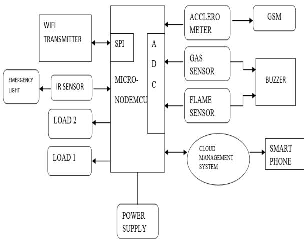
Home automation the use of MQTT is supplied for sending/receiving records from the sensor. For this ATMEGA328 is used as a gateway for getting access to the records from the sensor which person can manipulate their domestic equipment the use of the web-primarily based totally interface. In domestic automation the use of cellular is stated wherein gadget is designed the use of WiFi.
