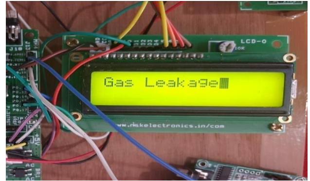
Fig 5.4 Gas leakage indication via GSM
