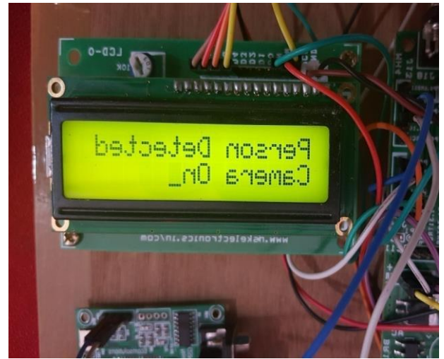
Fig 5.10 Turning On camera when person detected
