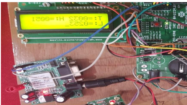
Fig5.3 Different average values of temperature (T), Light (L), and humidity (H).
