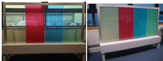
Fig. 3. Examples of colours available in smart glass(PDLC) [3]
