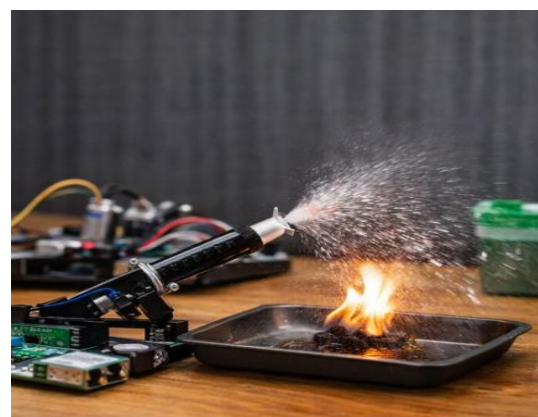
Fig 6.2 Fire suppression using a water pump
