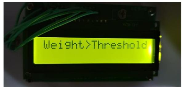
Figure 4: When the weight measured is greater than the threshold, the alert system is activated.
