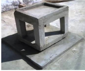
Fig. 2. Prototype model of spring Base isolator structure
