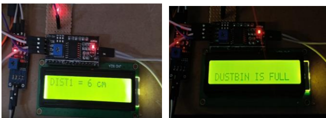
Fig. 8 LCD display of dustbin full
