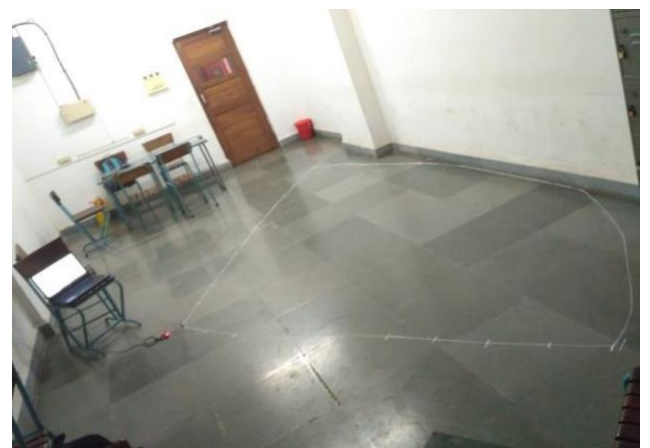
Figure 10: Determination of the range of the PIR sensor through experimental set up
