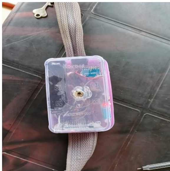
Fig. 3 Top view of developed smart collar system
