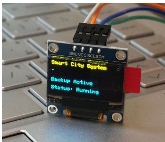
Fig. 5. OLED display showing successful switching to the backup network during testing.
