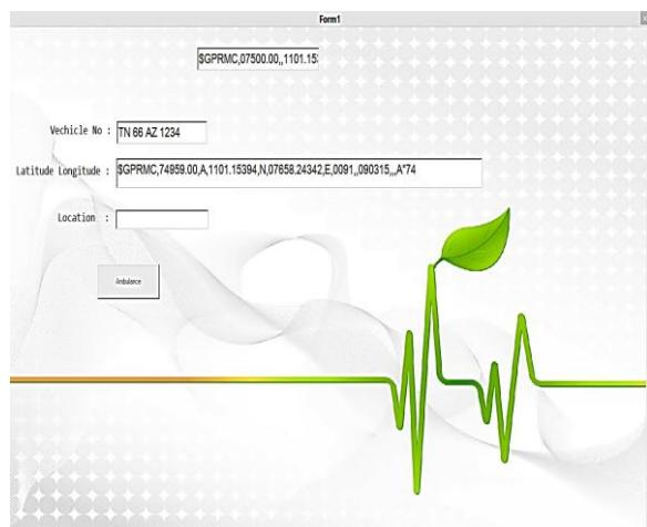
The location can be obtained by decoding the magnitude of latitude and longitude using GPS decoder after which the notification regarding the accident is intimated to ambulance automatically. The front-End of VB (II) appears as shown in the figure.
