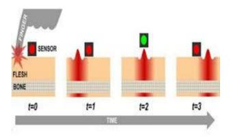
Finger impacts displace the skin, creating transverse waves. The sensor is activated as the wave passes underneath it.
