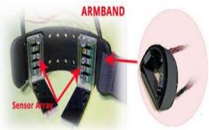
Inside the Skinput armband is a pair of sensor arrays, each consisting of five sensors. When the armband is wrapped around your arm, one array sits on top of your arm and the other below it, giving the sensors the widest range of useful data.
