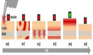
Finger impacts create longitudinal waves that cause internal skeletal structures to vibrate.
