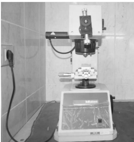
Figure 4. Vickers micro-indentation hardness
