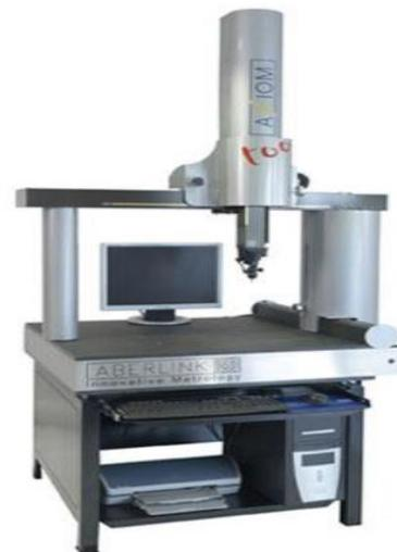
Figure 6. Coordinate measuring machine (CMM)
