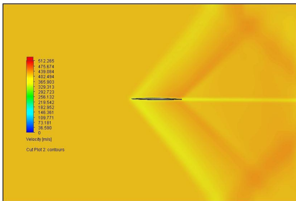
Fig.14. c) Velocity Contours at wing section C-C
