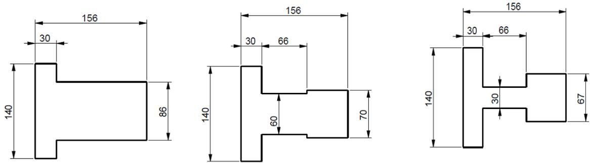
Figure 3.13 Section at pass-12    Figure 3.14 Section at pass-13    Figure 3.15 Section at pass-14
