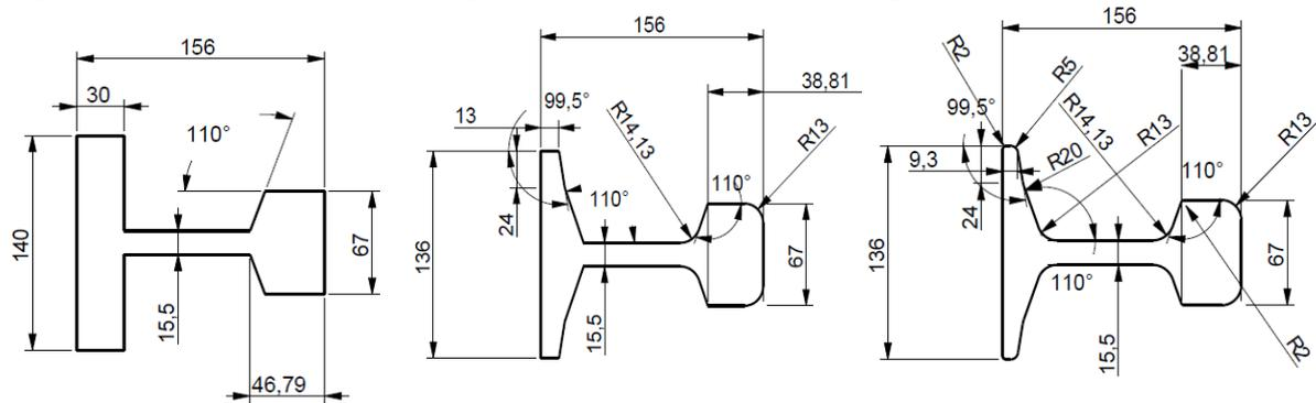
Figure 3.16 Section at pass-15    Figure 3.17 Section at pass-16    Figure 3.18 Section at pass-17
