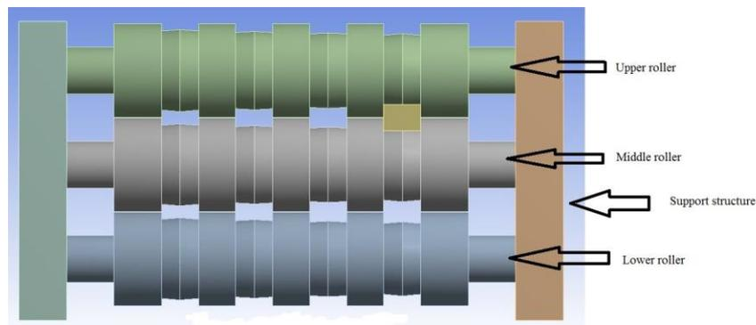
Figure 4.1 Rolling stand sample and its components
