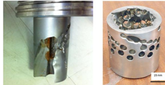
Fig. 4 Sand erosion damage to flow control part
