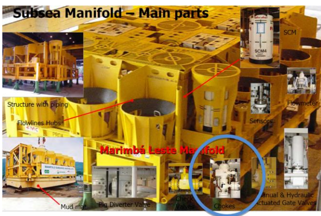
Fig. 2 Manifold System comprising equipment's
