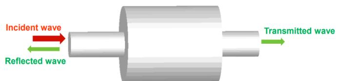
Fig. 10. Illustration of transmission loss in a muffler.
