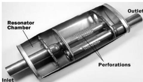
Fig. 2. Reactive Muffler. (3)
