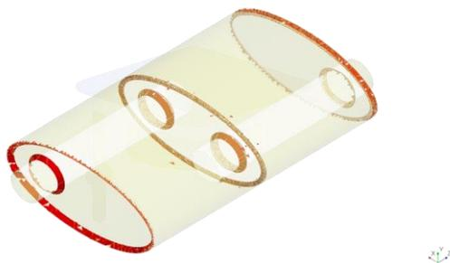
Fig. 16. Welded regions on solid muffler.
