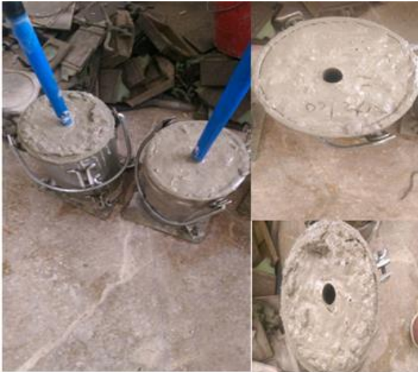
Figure 6: Samples with PVC immediately after preparation and without PVC pipe after setting.
