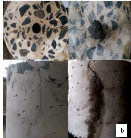
Figure 10: RS samples in (a) and VIB samples in (b) showing top surfaces and side cracks
