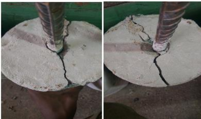
Figure 3: VIB concrete samples showing failure patterns and some visible cracks
