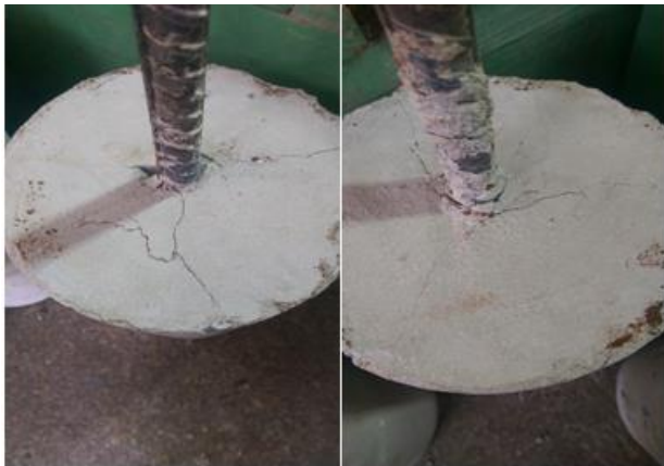
Figure 2: RS concrete samples showing visible cracks after the test
