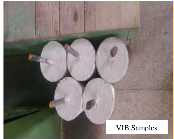
Figure 1: Concrete cylindrical samples (RS and VIB) after 14 days of curing.
