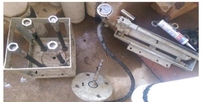
Figure 5: Hydraulic concrete cracking machine
