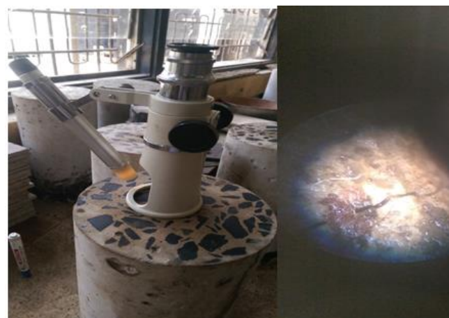
Figure 9: Observation of crack widths using crack meter
