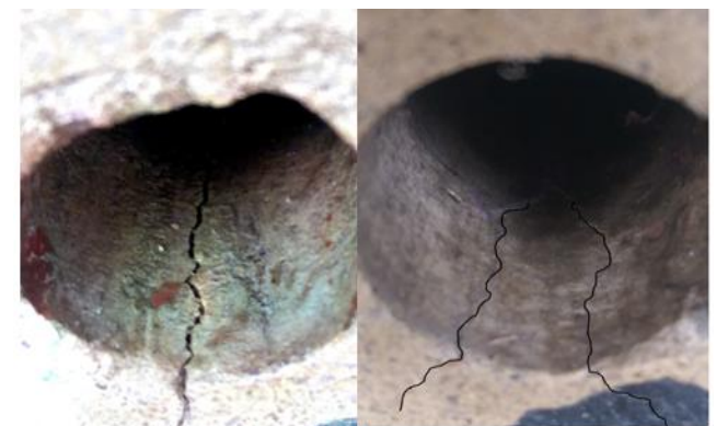
Figure 11: RS sample general pattern for both 7&28 days and VIB inner layer cracks
