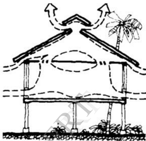
Figure 23: Suggested modifications for causing internal air flow
