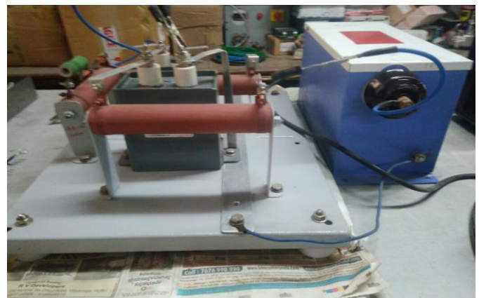
Fig. 4. Arrangement of components for generating lightning impulse
