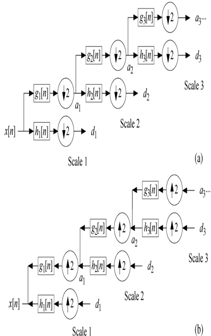
Fig. 2. Procedure of WT-based MRA (a) Decomposition (b) Reconstruction
