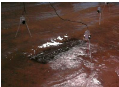
Fig 9. Breakwater in zero submerged condition
