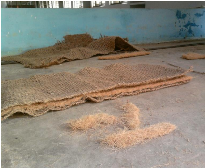
Fig 3. Coir fibre mat used as filter media
