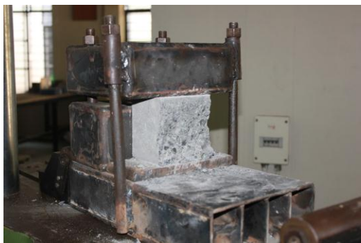
Fig. 5. Typical view of the failure plane
