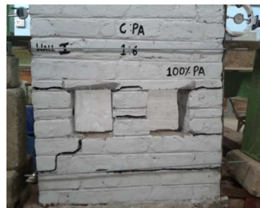
Failure of wall specimens C:S 1:6 single and double opening
