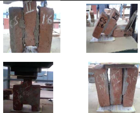
Fig 6 Failure pattern of brick triplets with C : S 1 : 6 mortar
