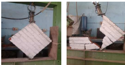
Fig 9. Experimental set up and Failure of the wallettes
