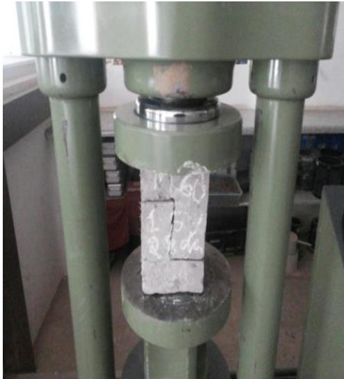
Fig.1: Typical Dimensions of Push-off Specimen Used and a Failed Specimen under Loading
