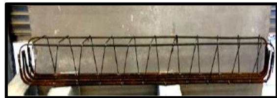
Fig.2 Continuous rectangular spiral reinforcement
