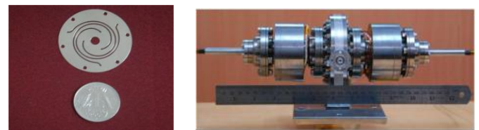
Fig 7 (a, b): Flexure Bearing and Dual-ported linear compressor developed in IISc [7]
