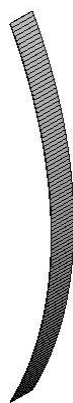
Fig. 11 The solid model of a cantilever beam spring with right circular undeformed shape.
