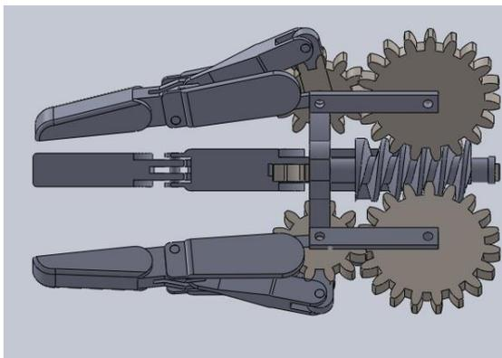
Fig.10-assembly of gripper in CAD software
