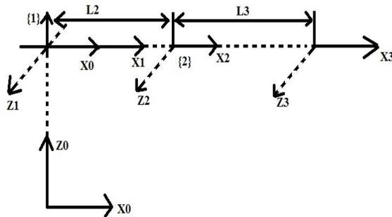
Fig.20. Frame diagram
