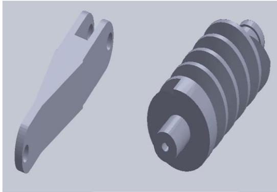
Fig.9 Link and worm gear
