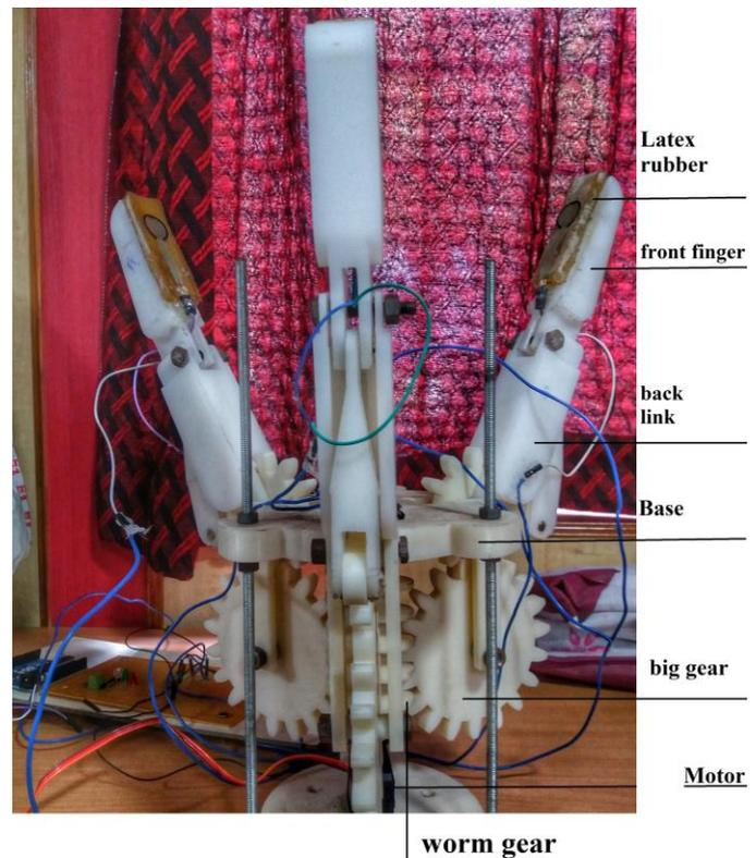
Fig.18 Three finger gripper
