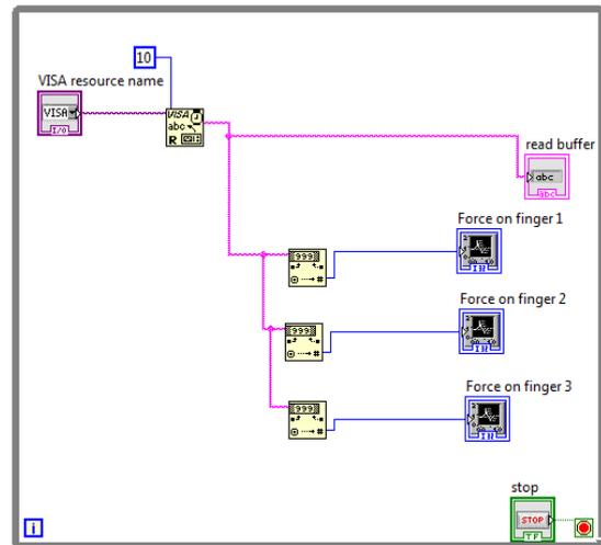
Fig.17. LAB view block diagram for obtaining force measurement
