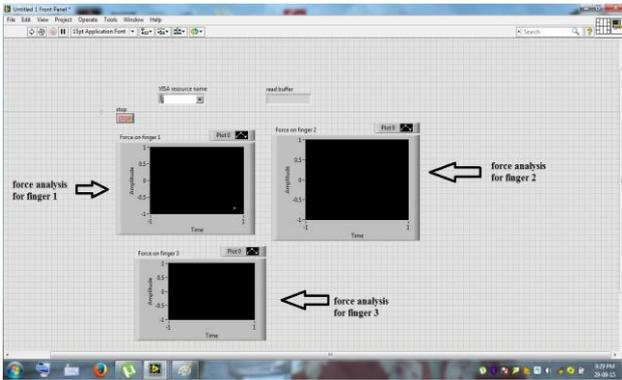
Fig. 19. Sensing the force from each finger using LAB view
