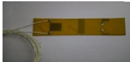
Fig.1(c). The sensor fabricated on PCB (Without paryline coated).
