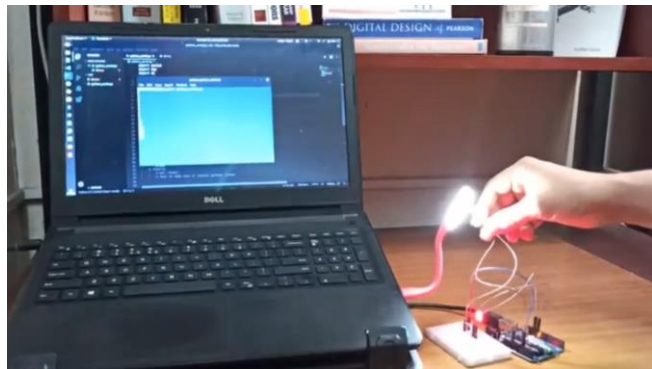
Fig 4: Working of the LDR portion of the proposed system. (a). When light is very far from LDR (b). When light is at an optimum distance from LDR (c). When light is very close to LDR.
