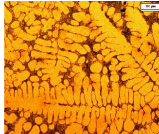
Fig 5.1 No shear LM25 cast in sand mold show in dendritic morphology of primary \alpha -Al (bright phase)
