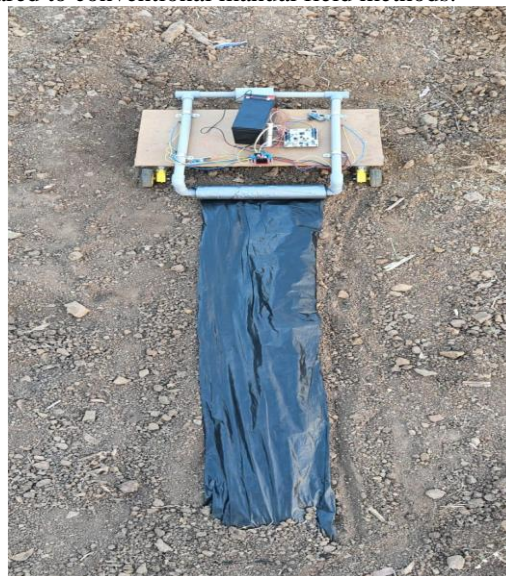
Fig.3 Actual testing in farm with robot
