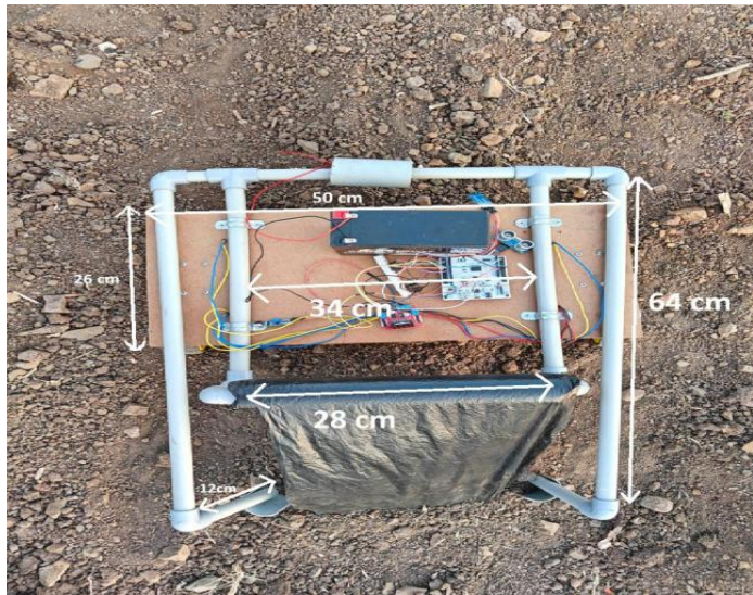
Fig.1 Agricultural robot with basic dimensions
