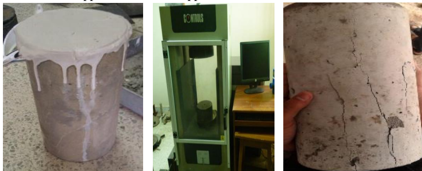
Crack introduction using compression testing machine
