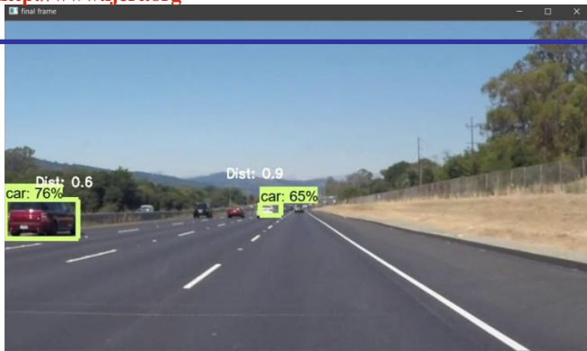
Fig. 3. YOLO Algorithm making predictions on the input feed.
