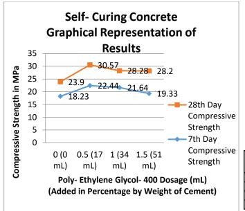
From the result, we can say that by 0.5 % addition of PEG the increase in the compressive strength is 27.9 % i.e. from 23.9 MPa to 30.57 MPa. But for 1% and 1.5 % of PEG-400, there is only an increase of 18.32 % in strength.
