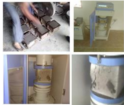
Fig2: Various stages of Cube testing
