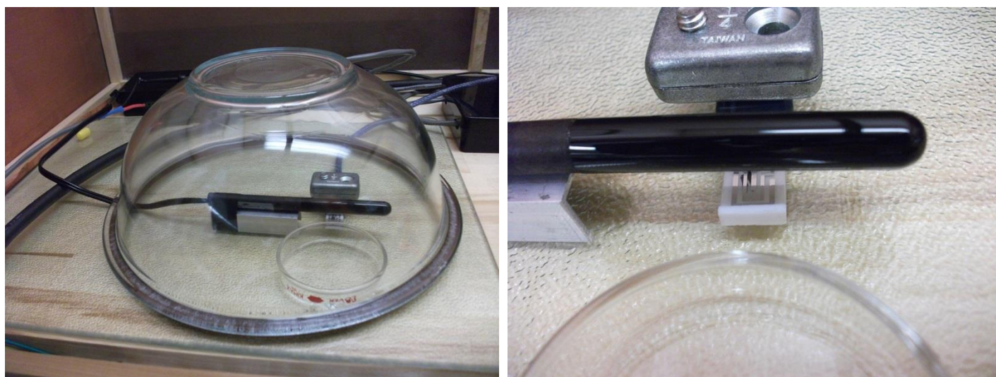
Figure 2. Experimental setup with the CoIDAE next to a petri dish containing the liquid PET that evaporates inside the glass chamber. The UV lamp for cleaning the sensor is also shown above the CoIDAE.
