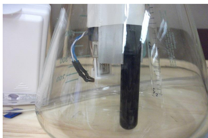
Figure 3. Experiment setup with a \text{TiO}_2 -CoIDAE contained within a sealed glass Erlenmeyer chamber. Also contained within this chamber is the UV light source (365nm Pen Ray, \sim 3\text{-}5 \text{ mW/cm}^2 ), a hygrometer sensor, and a temperature sensor. In photo to the right, one can see: temperature & hygrometer sensors (behind the CoIDAE), CoIDAE, UV lamp, and glass intake tube.
