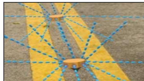
Fig. 8. Water flows from studs and clean the road
