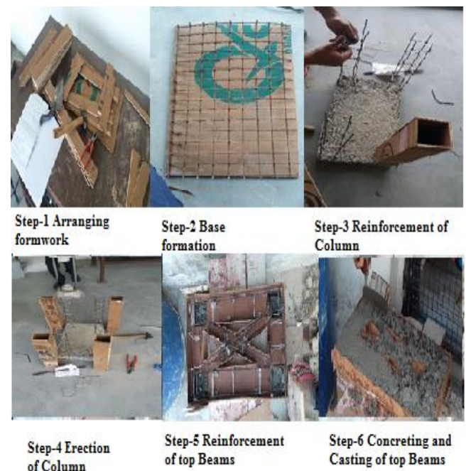
Fig-1 Different construction phase of testing model
