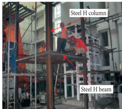
Fig. 10. The steel frame composed of steel H beams and steel H columns.
