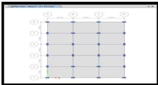
**Step 4.4:** Go to the “Base Plan” and select all the slabs and Delete them and see that modify storey is kept to “One Storey” only.
