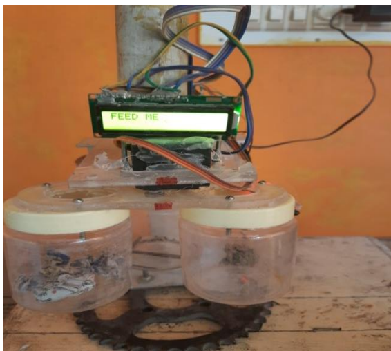
Figure 3 the working model of the Segregating the Waste Material using Rotating Model. This model has number of Sensors connected to the Arduino UNO to the Rotating table and also the LCD Display.
